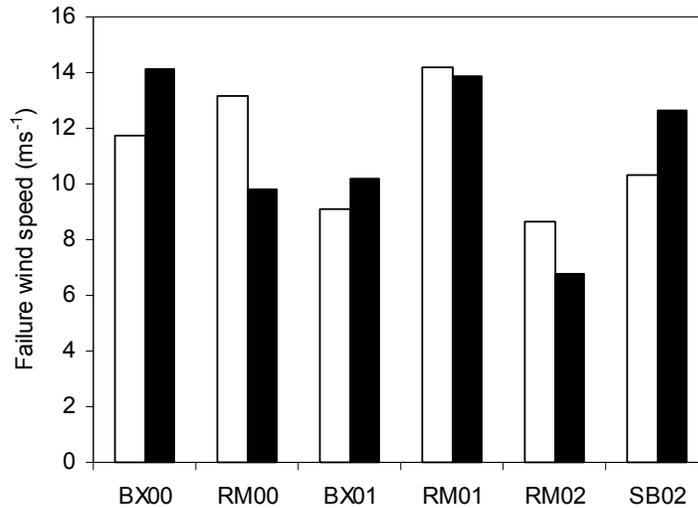
Fig. 1.2. Average stem failure wind speed (open bars) and root failure wind speed (closed bars) for each site season. Interaction SED =  $0.833 \text{ ms}^{-1}$  (15 df).
