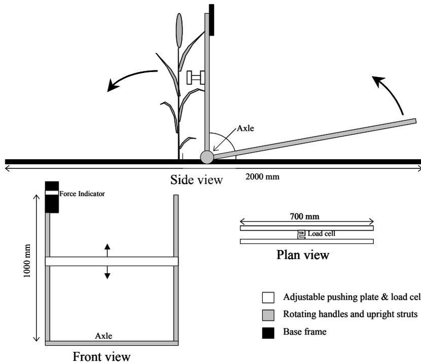
Fig. 2.1. Diagrams of the lodging instrument from the side, front and top.
