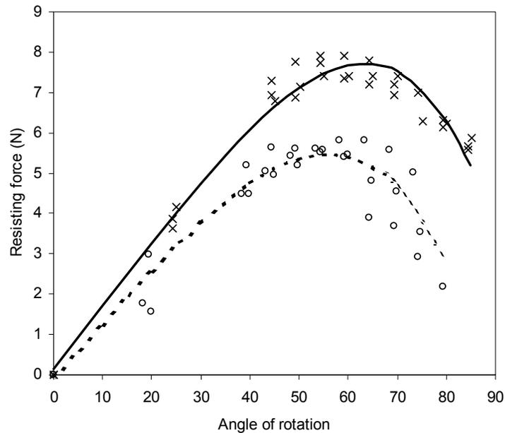
Fig. 2.2. Rotational resistances for a row of shoots in dry soil at SB for Equinox (—) ( $y = -14.55 + (14.70 - 0.127x) \times (1.019^x)$ ;  $R^2=0.97$ ) and Rialto (---) ( $y = -14.87 + (14.65 - 0.137) \times (1.019^x)$ ;  $R^2=0.91$ ). Critical exponential curves were fitted to data which was recorded using Method 1.
