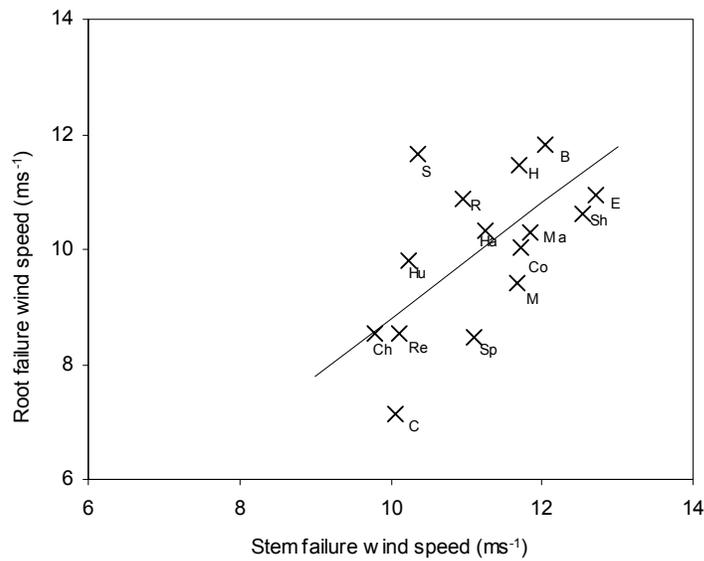
Fig. 1.3. Stem failure wind speed plotted against root failure wind speed for 15 winter wheat varieties; B-Buster, C-Cadenza, Ch-Charger, Co-Consort, E-Equinox, Ha-Harrier, H-Hereward, Hu-Hussar, Ma-Madrigal, M-Mercia, Re-Reaper, R-Rialto, S-Savannah, Sh-Shamrock, Sp-Spark. The mean difference between the stem and root failure wind speeds is represented by  $y = x - 1.2$  (—). The SED for the interaction between type of failure and variety =  $0.594 \text{ ms}^{-1}$  (162 df).
