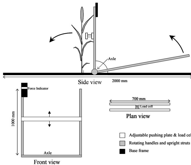
Fig. 3. Diagrams of the lodging instrument from the side, front and top.
